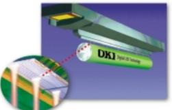
The rock-solid OKI Digital LED printhead utilizes a stationary array of pulsing light-emitting diodes (detail) to create high-resolution text and graphics.
